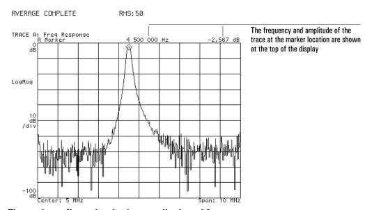
The marker reflects the absolute amplitude and frequency
