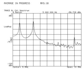
The spectrum with averaging turned on. Note existence of three components.
