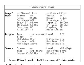
State summaries provide a quick view of the instrument setup parameters
