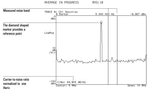
Now the value indicated in the lower left corner of the display reflects the difference between the marker level at the carrier peak and the noise-power within the band markers normalized to one Hertz bandwidth.
