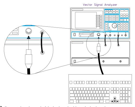
**3** Connect the other end of the keyboard cable to the keyboard.
