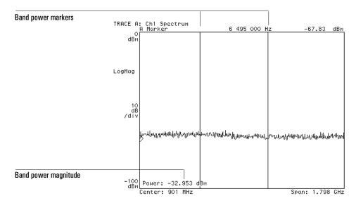
In this example you are measuring the power of the analyzer's noise floor within a defined band. The value displayed in the lower left corner of the display reflects the total power within the frequency band encompassed by the markers. The grid lines have been turned off to highlight the band power markers.
