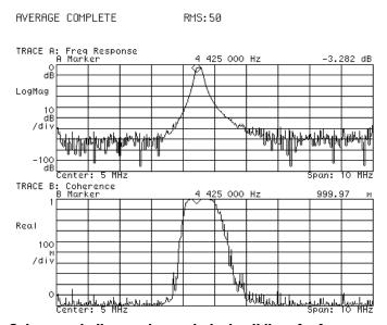
Coherence indicates the statistical validity of a frequency response measurement
