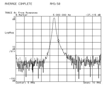
Frequency response data displays the output of a device-under-test divided by the input
