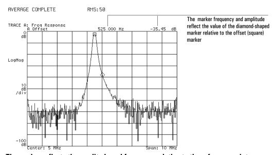
The marker reflects the amplitude and frequency relative to the reference point
