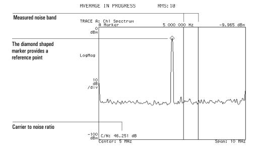
The value indicated in the lower left corner of the display reflects the difference between the marker level at the carrier peak and the total noise within the band markers.
