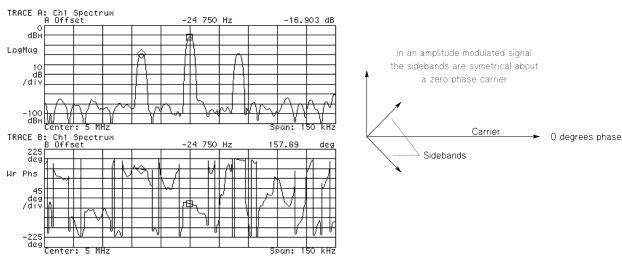
The phase values vary with each sweep but for an AM signal the average phase of the sidebands is equal to the carrier phase.
