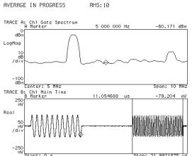
Spectrum (top trace) of the burst is derived by gating the time signal (bottom trace). The gate's delay and length are selected to encompass the burst signal (vertical markers show gate position). Note existence of the first spectral component in the left display and the existence of the other two components in the right display.
