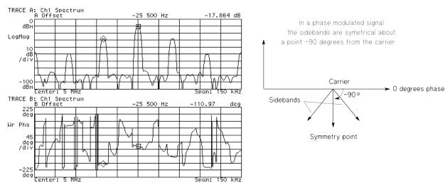
The phase values vary with each sweep but for a PM signal the average phase of the two sidebands is equal to -90 degrees from the carrier.
