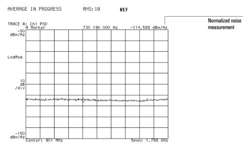
In this example you are measuring the noise-power of the analyzer's noise floor. The displayed marker value reflects noise-power normalized to a 1-Hz bandwidth.
